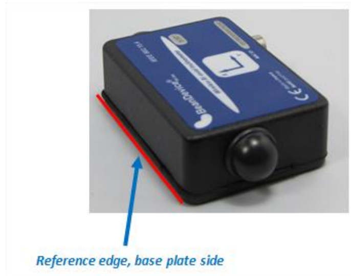
Figure 6: BeanDevice® mounting reference angle
