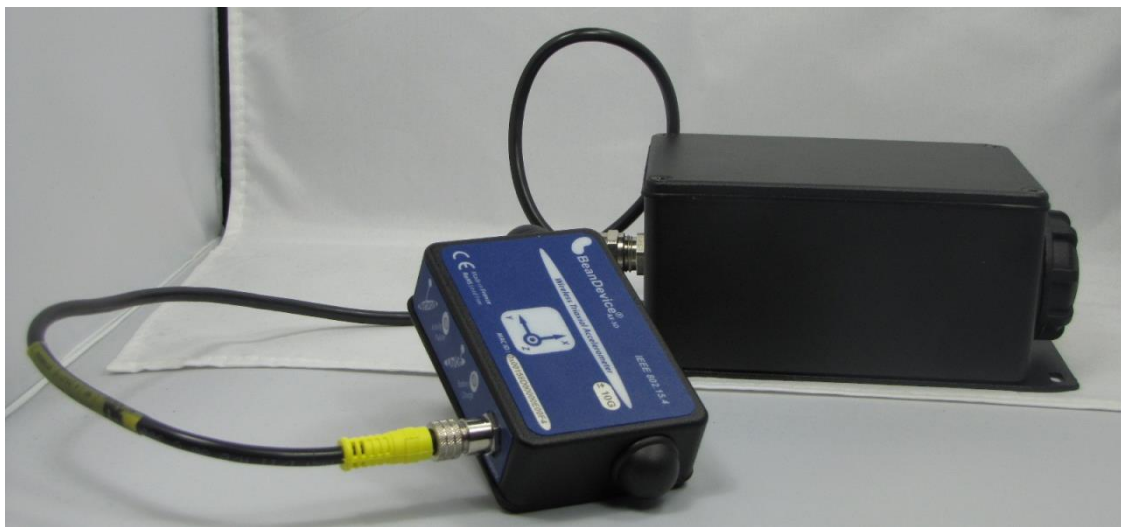
Figure 12: Changing the External Primary cell (connecting the BeanDevice®)
