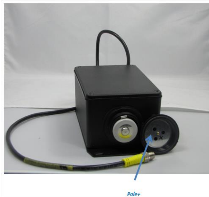
Figure 10: Changing the External Primary cell
