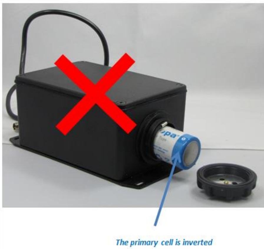
Figure 11: Changing the External Primary cell (wrong practice)
