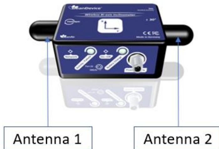
Figure 5: Antenna position on the BeanDevice AX-3D
